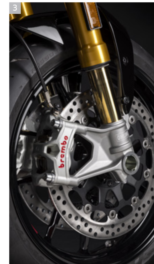
3 Radially mounted Brembo Stylema® monobloc 4-piston callipers
